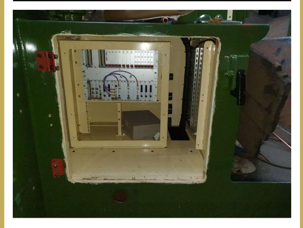
If you missed this week's update on the progress of the ETCS equipment being fitted onto *Tornado*, with the first components finding their home in the new locker in the tender,
